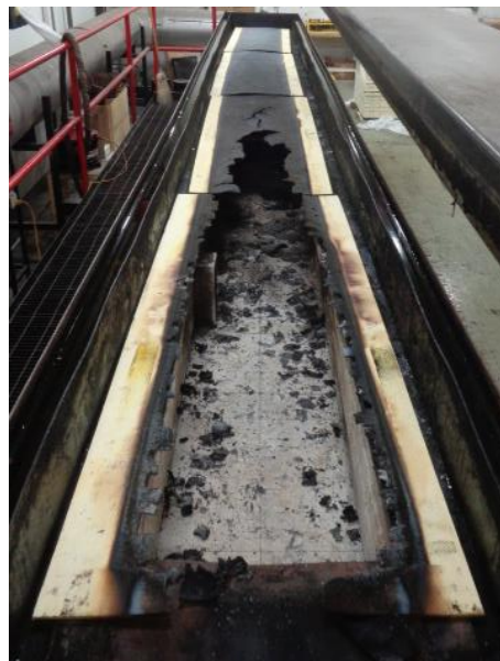
Photo No. 4 Exposed Surface of the Test Specimen (Post-test)
